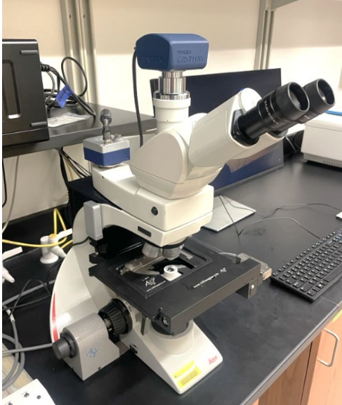
Leica DM2000 Brightfield; Upright BSBS 125 Jenoptiks Camera 5, 10, 20 and 40x
